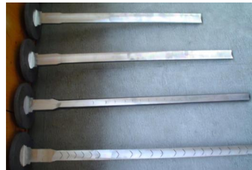
Fig. 1. Experimental chevron defects found in open-die extrusion process
